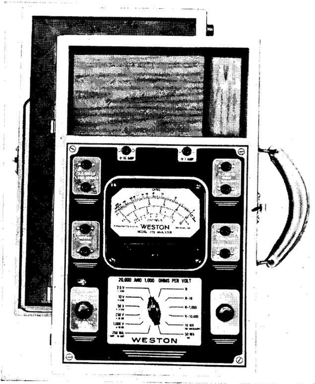
FIG. 4-1.—The Weston Model 772 multimeter.
