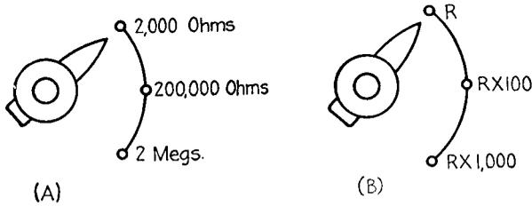
FIG. 4-15.—Typical ohmmeter range switches.
