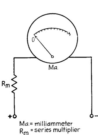
FIG. 4-2.—A basic voltmeter.
