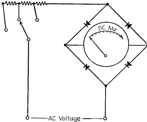
FIG. 4-12.—Typical multirange AC voltmeter.
