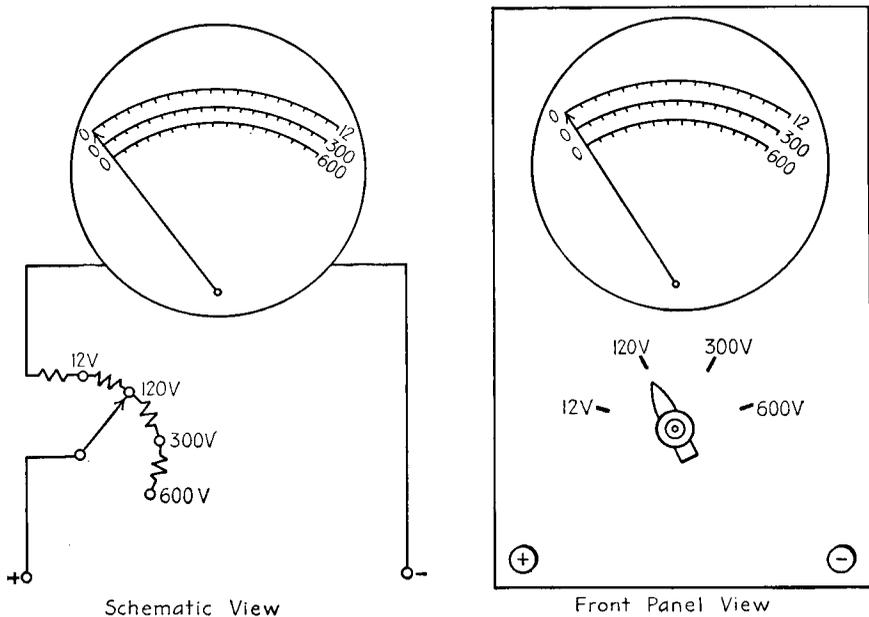
FIG. 4-5.—Multirange voltmeter showing range switch.
