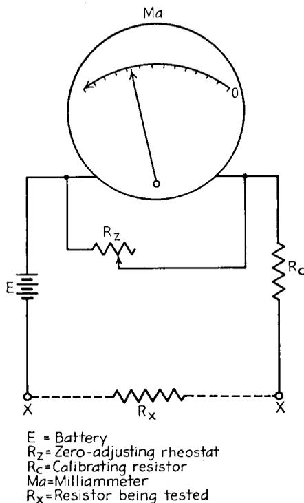
FIG. 4-13.—Basic ohmmeter circuit.
