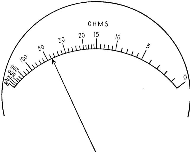
FIG. 4-14.—Typical ohmmeter scale.
