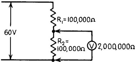
FIG. 4-9.—Measuring the voltage with a 20,000-ohms-per-volt meter.
