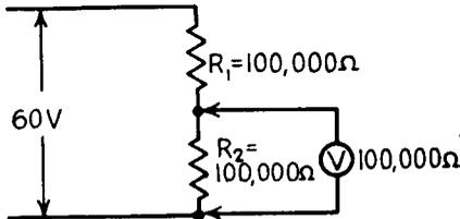
FIG. 4-7.—Measuring voltage with a 1,000-ohms-per-volt meter.
